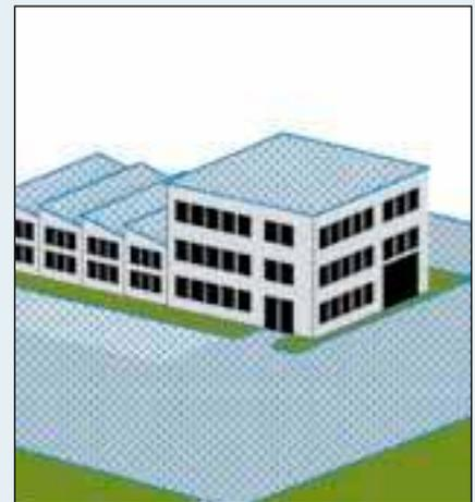
Surfaces of the connected buildings plus roof overhangs (independent of roof pitch) + other connected surfaces.
